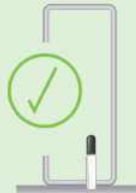
Screw located close to the web, ensuring a tight fix to the cladding
