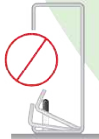
Screw located too far from the web, will cause bending of flange and a loose fixing of the cladding
