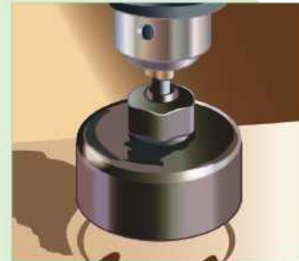
Hole forming (hole saw)
